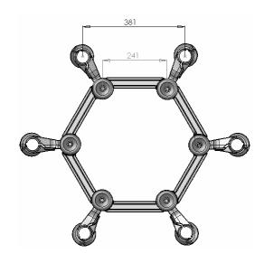
Six bundle spacer - Dampers are used to control aeolian vibration and conductor oscillation. Maintain conductor spacing and restore conductor spacing after a short circuit occurs.
