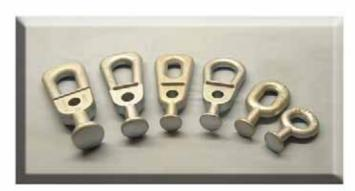
A range of ball ended fittings is available encompassing ball hooks, ball eye links, ball clevis and ball tongues. Ball and shank sizes range from 11mm. up to and including 28mm. with failing loads of between 20kN and 400kN.
