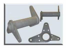
Yoke plates for all types of constructions and conductor configurations are available. These range from the simplistic 15/22 design rated at 70kN to the more complex designs for triple insulator strings and quad conductors rated at 800kN.
